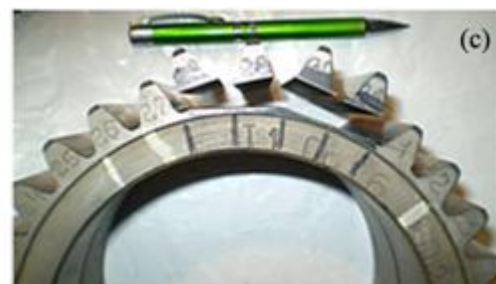
Fig. 10. Grounded gear before (a) and after (b, c) cutting off the four teeth
