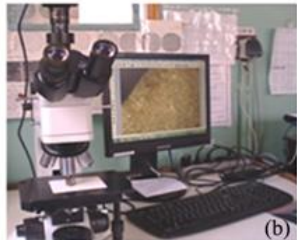
Fig. 13. Hardness measurements both on PMT-3 instrument (a) and microscope Altami MET-5 (b)
