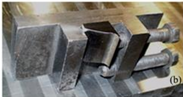
Fig. 11. Samples prepared from fragment teeth when the sample is clamped in the fixture (a) and installed onto the machine table (b)
