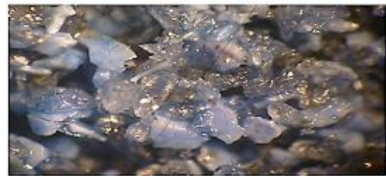
Fig. 4. A fragment of the real surface of a highly porous grinding wheel obtained for the wheel specifications WG946Hs12Vs (a) and 3SG46Hs12Vs (b)
