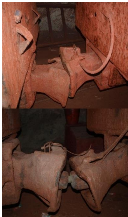
Fig. 1. Photographic evidence of conditions of drawbars of VG-4.5 cars (for two extreme positions)
