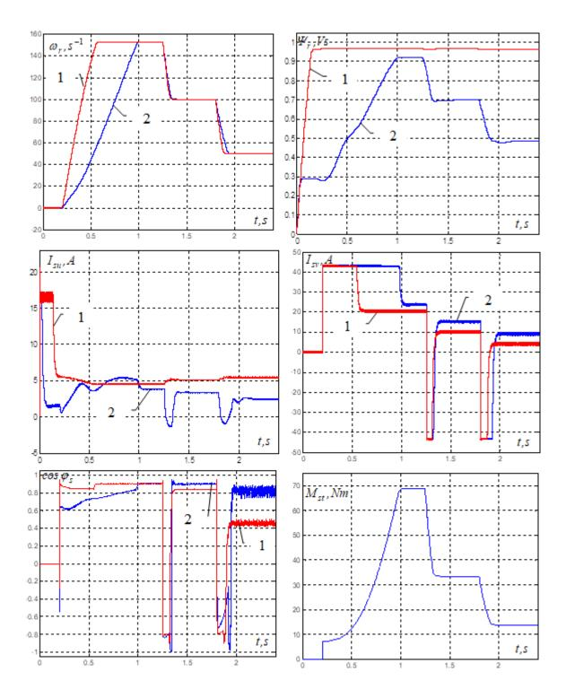
Fig. 5. Graphs of transients in an asynchronous electric drive with vector control: 1 – system with stabilization of magnetic flux at nominal level;
