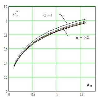
Fig. 3. Dependences of extreme values  $\Psi_r$  for  $Q_s$  from the moment of loading  $\mu_{st} = M_{st} / M_n \text{ at different speeds}$ Source: compiled by the author
