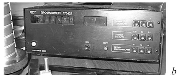
Fig. 10. Profilometer for measuring surface roughness: setting (a) and measuring part (b) Source: compiled by the author
