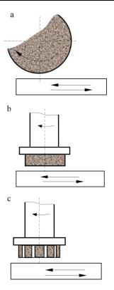
Fig. 3. Common schemes of continuous (a, b) and intermittent (c) grinding Source: compiled by the author
