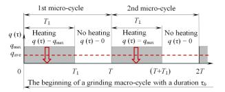
Fig. 1. Pulsating heat flux  $q(\tau)$ :  $0T_1$  and  $T_1T$  are time intervals of "heating" and "no heating" Source: compiled by the author
