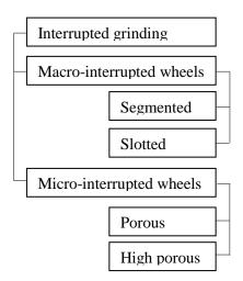
Fig. 2. Interrupted grinding wheels classification based on the wheels geometrical parameters Source: compiled by the author
