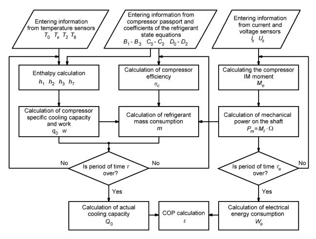
Fig. 8. Algorithm for SRU energy efficiency estimation Source: compiled by the author
