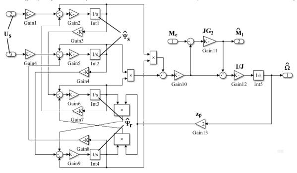
Fig. 6. The simulation model of the IM full order state observer Source: compiled by the author
