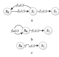
Fig. 1. Graph example: a) original graph;b) equivalent transformation of parallel arcs;c) equivalent transformation of loop-arc
