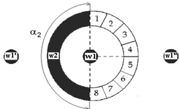
**Fig. 2. The calculation model of the toroidal CT**
