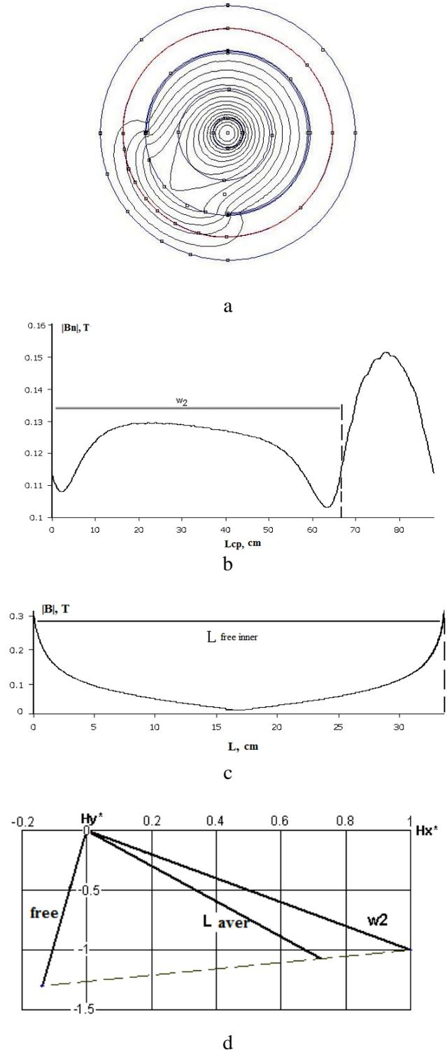
Fig. 5. The magnetic field at  $\alpha_2 = 270^\circ$
