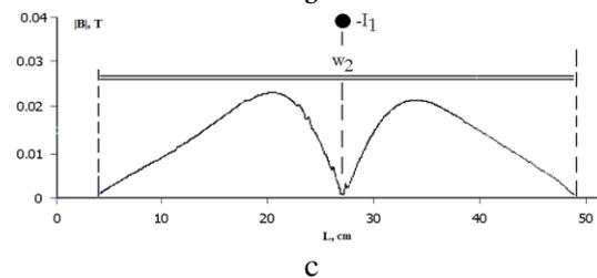
Fig. 7. The distribution of the magnetic field with the location of the reverse wire from the secondary winding side
