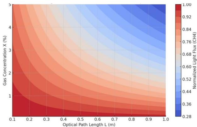
**Fig. 2. Dependence of  $CH_4$  light flux on concentration and optical path length**
