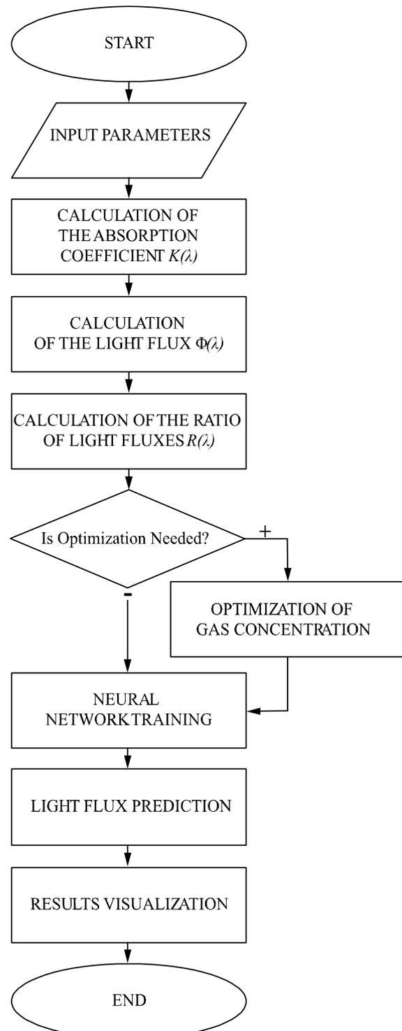
Fig. 1. Model operation algorithm
