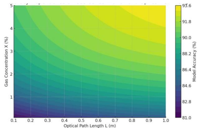
**Fig. 3. Model accuracy on gas concentration and optical path length**
