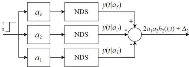
**Fig. 4. Structural scheme for computing the diagonal cross-section of the second-order transient characteristic using the compensation method with three test signals**
