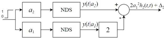
**Fig. 3. Structural scheme for computing the diagonal cross-section of the second-order transient characteristic using the compensation method with two test signals**
