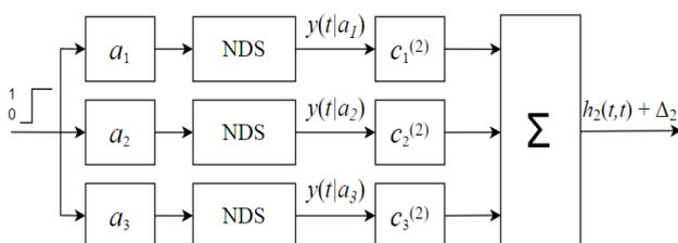
**Fig. 1. Structural scheme for computing the diagonal cross-section of the second-order transient characteristic using the approximation identification method**
