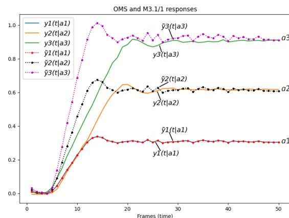
**Fig. 10. Responses of the EMS and the model M3.1 built using test signal with amplitude  $a_1$**
