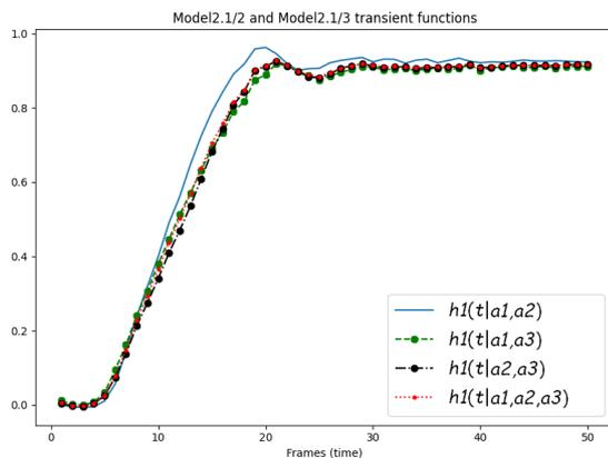
**Fig. 8. Transient characteristics of the EMS models M2.1/2, built using test signals with amplitudes:  $a_1$  and  $a_2; a_1$  and  $a_3; a_2$  and  $a_3;$  and M2.1/3**
