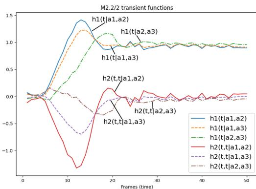
**Fig. 11. Transient characteristics of the first-order and diagonal cross-sections of the second-order of the EMS, models M1.2/2 and M2.2/2**
