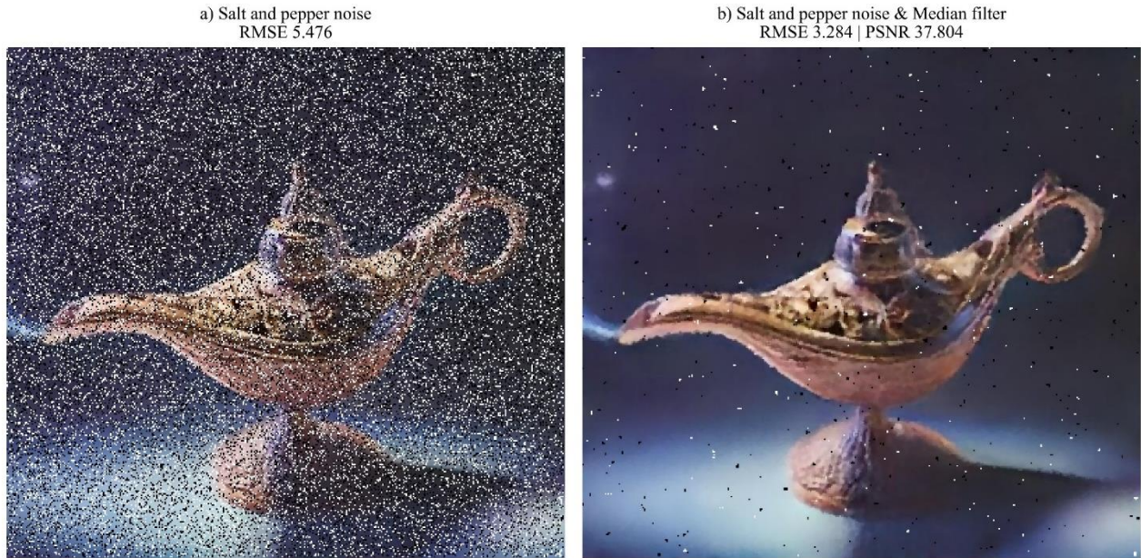
Fig. 3. Metrics of a median filter applied to noisy image
