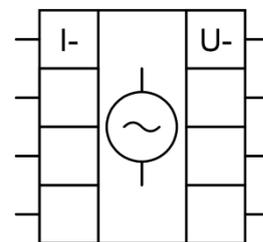
Fig. 9. The symbol for the block modeling of the alternating current voltage power source
