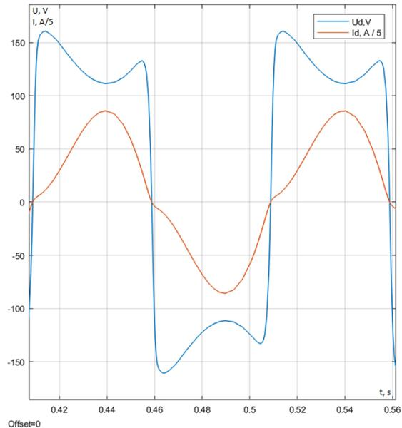
**Fig. 16. The dependency of voltage  $u_d$  and current  $i_d$  of the electric arc on time,  $f = 10 \text{ Hz}$**
