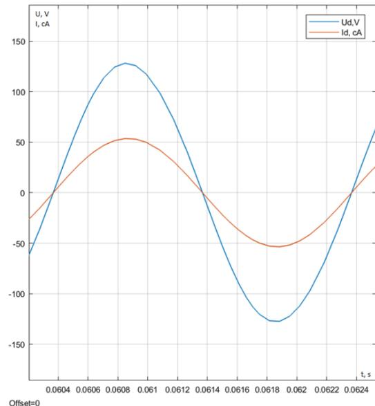
**Fig. 24. The dependency of voltage  $u_d$  and current  $i_d$  of the electric arc on time,  $f = 500$  Hz**
