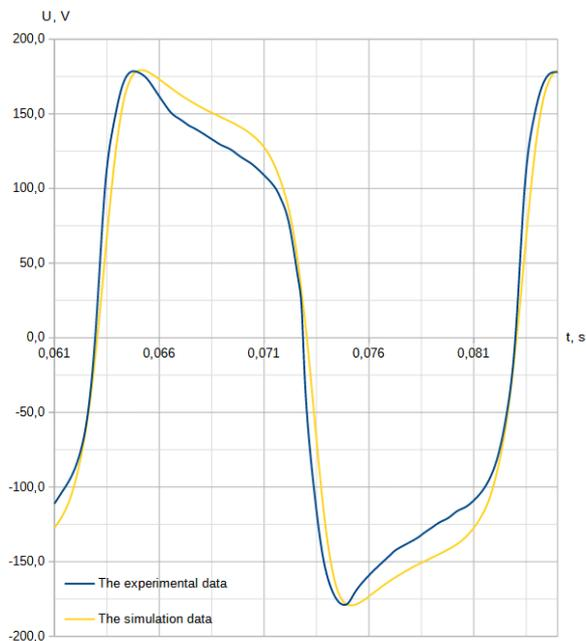
**Fig. 11. The voltage dependency  $u_d$  of the electric arc over time,  $f = 50$  Hz**
