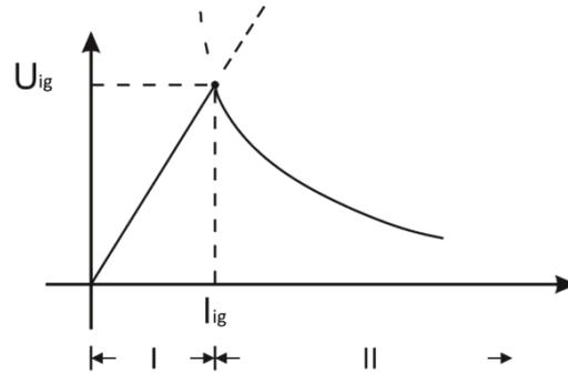
Fig. 4. Static voltage-ampere characteristic of an electric arc
