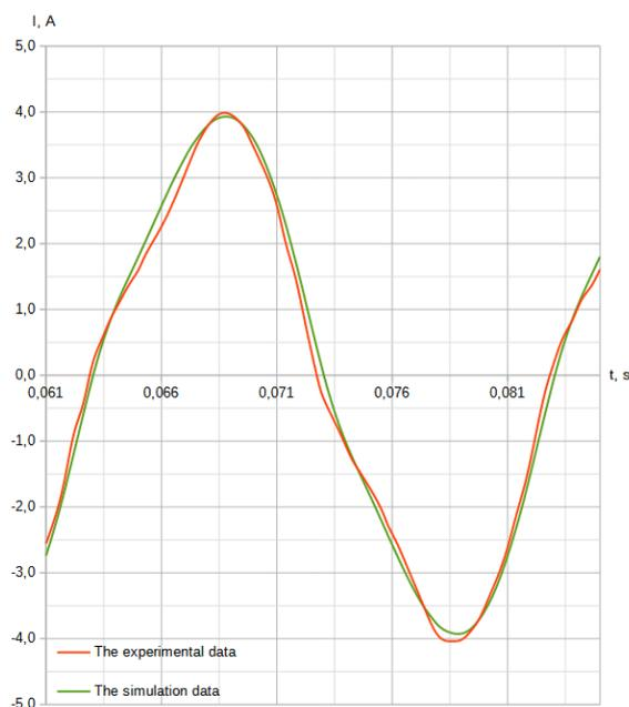
**Fig. 12. The current dependency  $i_d$  of the electric arc over time,  $f = 50$  Hz**
