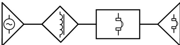
Fig. 3. The energy path diagram of the electric arc
