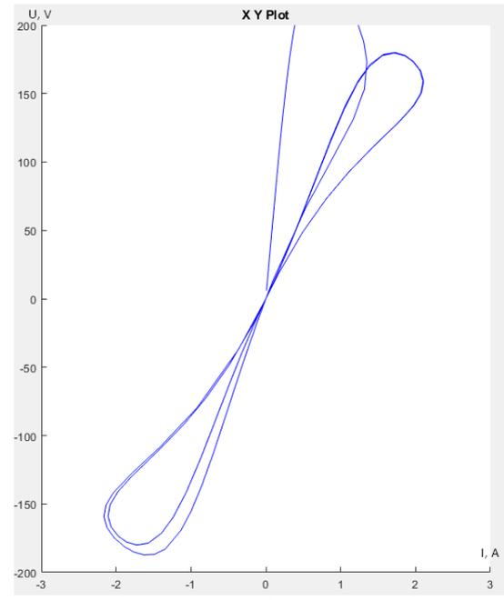
**Fig. 23. The dynamic current-voltage characteristic of the electric arc,  $f = 100$  Hz**
