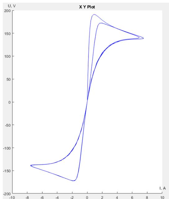
**Fig. 19. The dynamic voltage-ampere characteristic of the electric arc,  $f = 25$  Hz**
