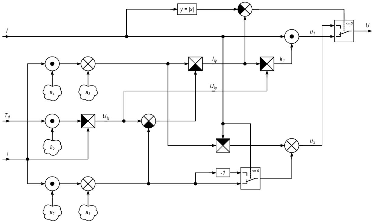
Fig. 6. The visual-block modeling of the electric arc
