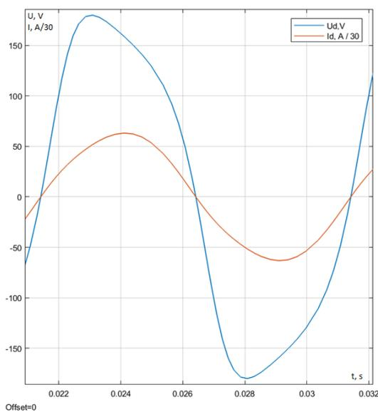
**Fig. 22. The dependency of voltage  $u_d$  and current  $i_d$  of the electric arc on time,  $f = 100$  Hz**
