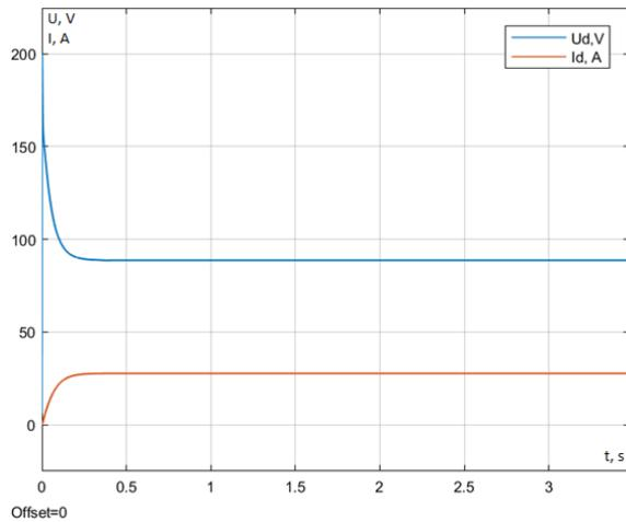
**Fig. 14. The dependency of voltage  $u_d$  and current  $i_d$  of the electric arc on time under direct current**
