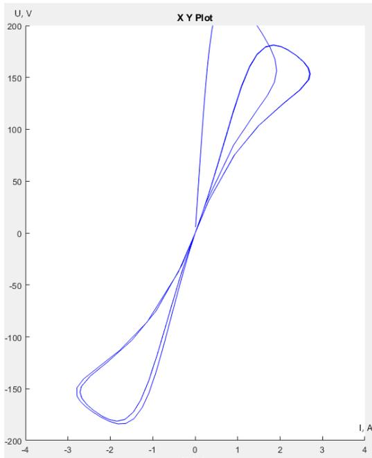
**Fig. 21. The dynamic voltage-ampere characteristic of the electric arc,  $f = 75$  Hz**
