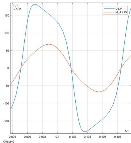
**Fig. 20. The dependency of voltage  $u_d$  and current  $i_d$  of the electric arc on time,  $f = 75$  Hz**
