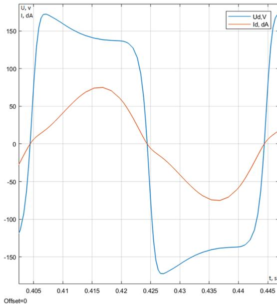
**Fig. 18. The dependency of voltage  $u_d$  and current  $i_d$  of the electric arc on time,  $f = 25$  Hz**
