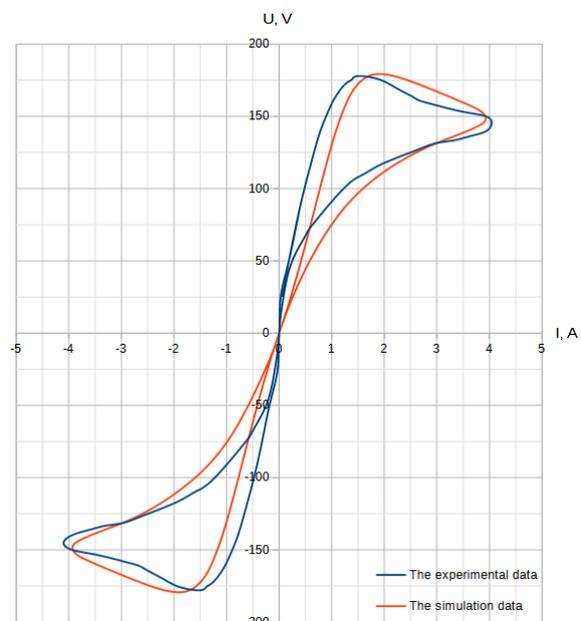
**Fig. 13. The dynamic current–voltage characteristic of the arc for  $f = 50$  Hz**
