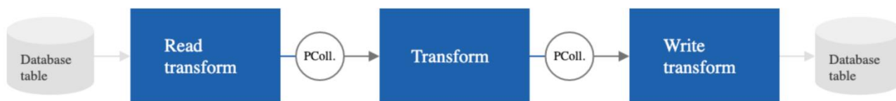
Fig. 3. Linear conveyor with sequential transformations
