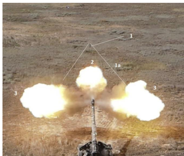
Fig.1. Muzzle ejection formed when firing from a 152 mm gun 2A36 “Hyacinth-B”[10]: 1 – projectile; 1a – mach cone accompanying the projectile; 2 – frontal ejection of powder gases; 3 – side ejection of powder gases through the holes of the compensator (muzzle brake ) tools
