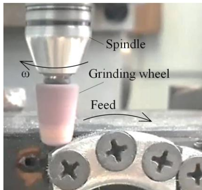
Fig. 12. Contour grinding with infinitesimal tool pressure (nanotechnology)
