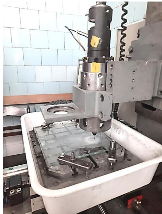
Fig.8. CNC mechatronic technological system based on AMM module
